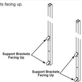
2. Attach a side bracket (3) to each upright using a 5/16"-18 x 2" capscrew (6) and a lock nut (8). The side brackets must extend to the outside of the upright.
